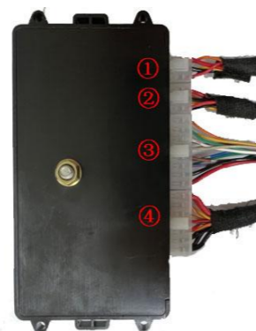
28. Insert the left and right strut wiring harnesses ① ②, lock signal harness ③, and power harness ④ into the ECU in sequence.
