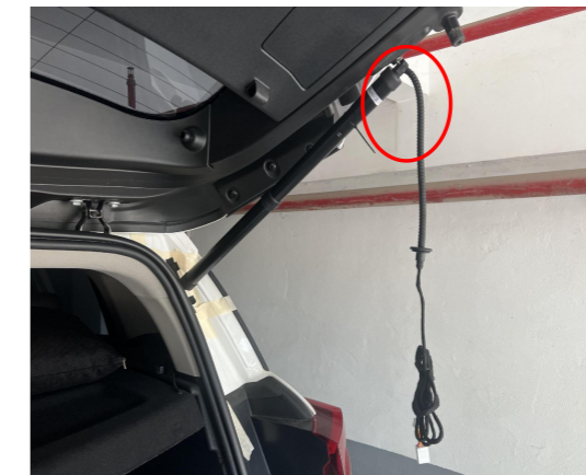
10. Install the electric struts, L on the left and R on the right (the first letter of the strut code).
