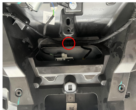
27. Remove the indicated cable clip.
