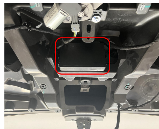
29. Fit the ECU into its bracket and tie the wiring harnesses to the original wiring harness.
