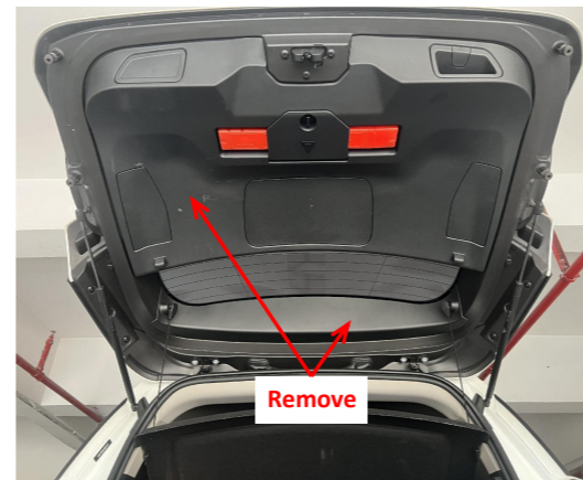
4. Remove the tailgate trim panels.
