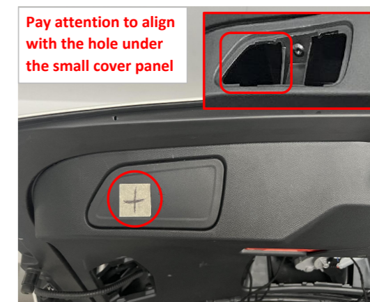
31. Stick the hole template to the indicated position and open a hole for the added tailgate switch.
