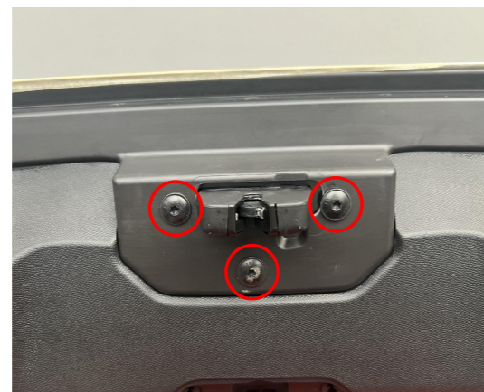
13. Remove the original latch.
