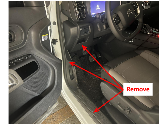
1. Remove the indicated driver's side trim panels.
