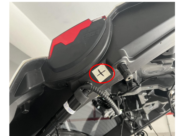
11. Drill a hole at the indicated position with a \varnothing 21 drill bit to allow strut wiring harness to pass through.
