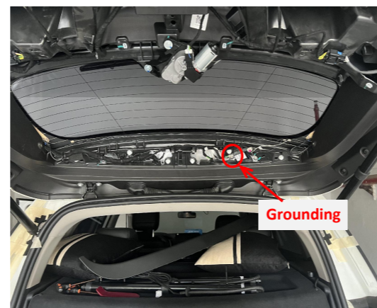
19. Ground at the indicated position of the tailgate.
