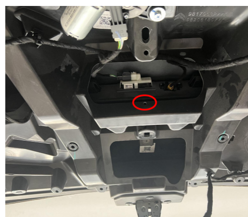
25. Drill a hole at the indicated position with a 6mm drill bit.
