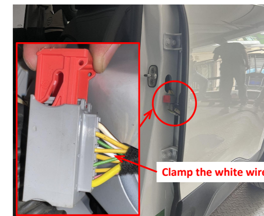
21. Clamp the white wire of the B-pillar signal plug to connect it to the orange wire of the power harness.
