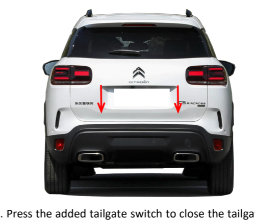
25. Drill a hole at the indicated position with a 6mm drill bit.
