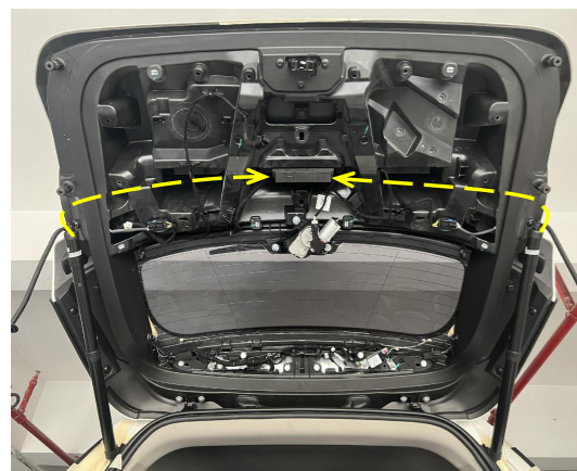
12. Thread the left and right strut wiring harness into the tailgate as indicated and plug the holes with rubber plugs.
