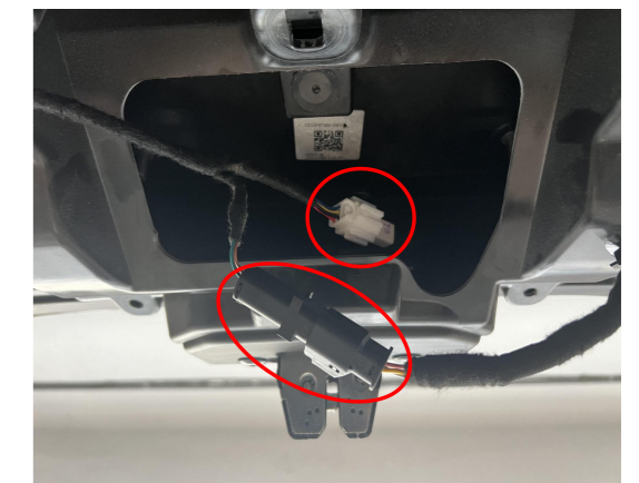
16. Connect the plugs of the lock signal harness to the plugs of the power latch.
