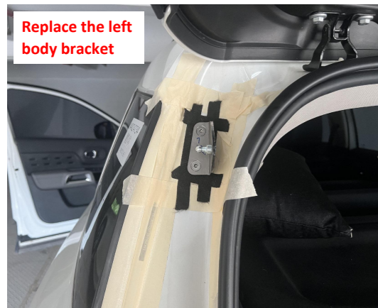
7. Replace the left body bracket.
