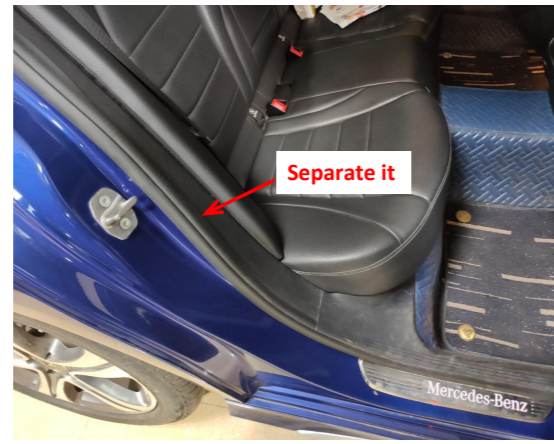
3. Remove the indicated trim panel.
