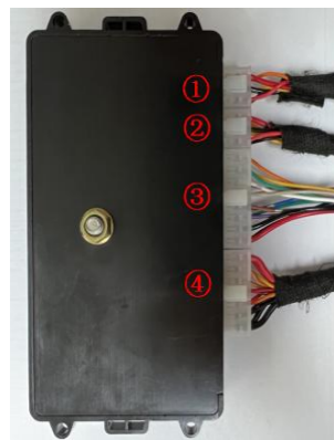
27. Insert the strut wiring harnesses ①②, lock signal harness ③, and power harness ④ into the ECU in sequence.
