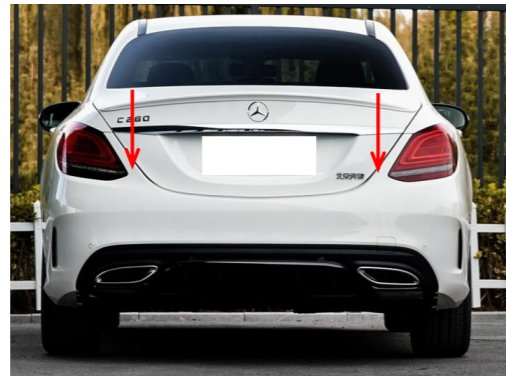
28. Manually close the tailgate until it touches the striker, then press the original tailgate switch button to open the tailgate. The system will complete initialization, and then test each function of the electric tailgate.
