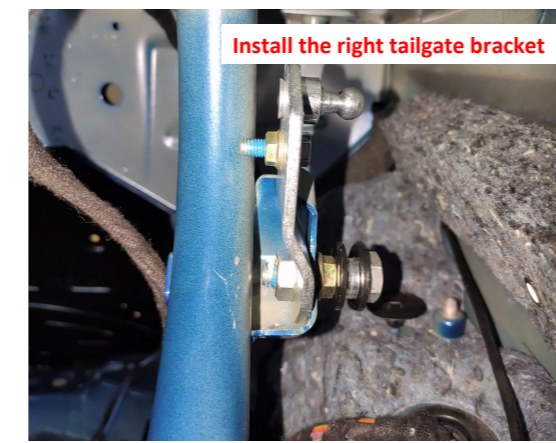
9. Install the right tailgate bracket on the right hinge.
