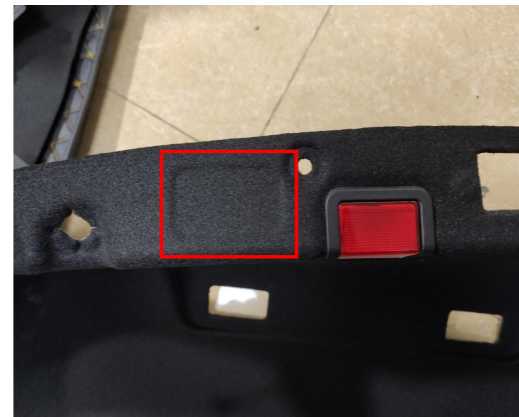
29. Stick the hole template to the indicated position on the tailgate trim panel.
