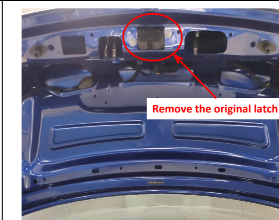
15. Remove the original latch.
