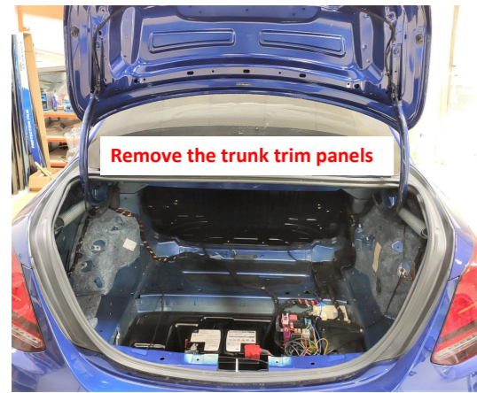
2. Remove the trunk trim panels
