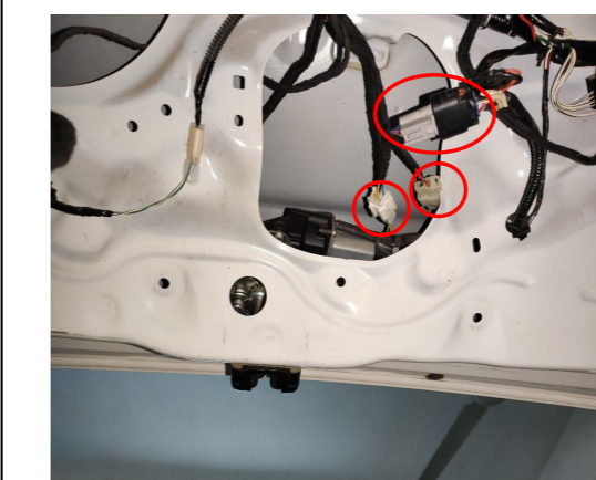
15. Connect the plugs of the lock signal harness to the plugs of the power latch
