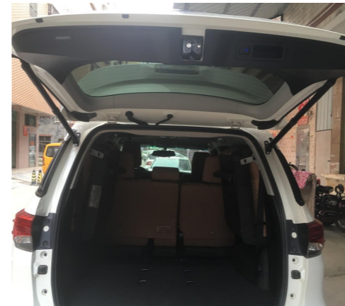
29. Reinstall all the trim panels and install the added tailgate switch.
