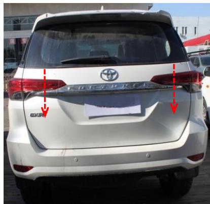
27. Press the added tailgate switch to open and close the tailgate once, the system completes initialization, and then test the functions of the electric tailgate.
