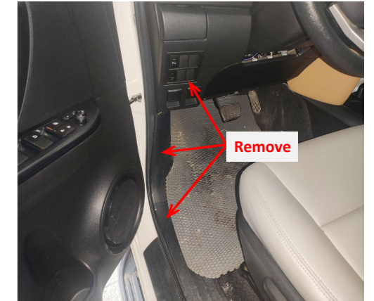
1. Remove the front left side trim panel, door sill panel and switch panel.
