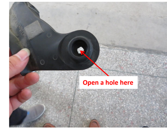
11. Open a hole at the indicated position of the rubber pads to allow the strut wiring harnesses to pass through.
