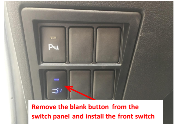
22. Remove the blank button from the switch panel, install the front switch, and connect to the plugs beside the switch for backlight.
