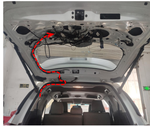
18. Route the power harness to tailgate.
